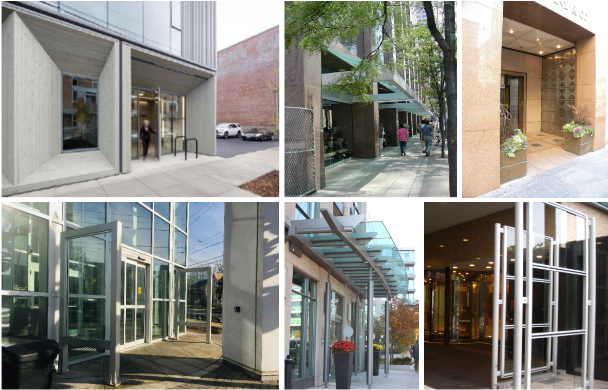
Image 4: Wind Control Features for Entrances
